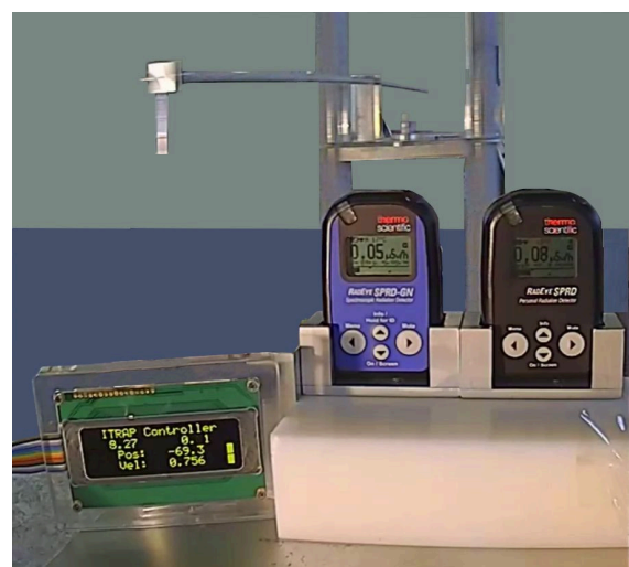
Fig. 1. RadEYE devices during testing. With the blue front the RadEYE SPRD GN with a CLYC crystal and with the black front the RadEYE SPRD equipped with a CsI crystal. The source at the extension bar is moving to the left. Below the source the control display is placed.
