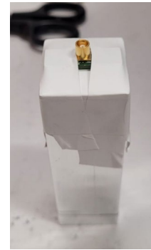
Fig. 7. CsI(Tl) crystal coupled to Hamamatsu S14160-6050HS SiPMs
