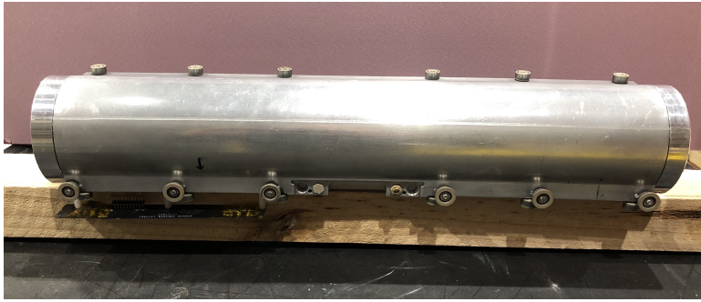
Figure 5. Left panel: The in-vacuum field camera, the so-called trolley. Right panel: The azimuthally averaged magnetic field contours \omega_p(x, y) overlaid with the azimuthally averaged muon distribution M(x, y) .
