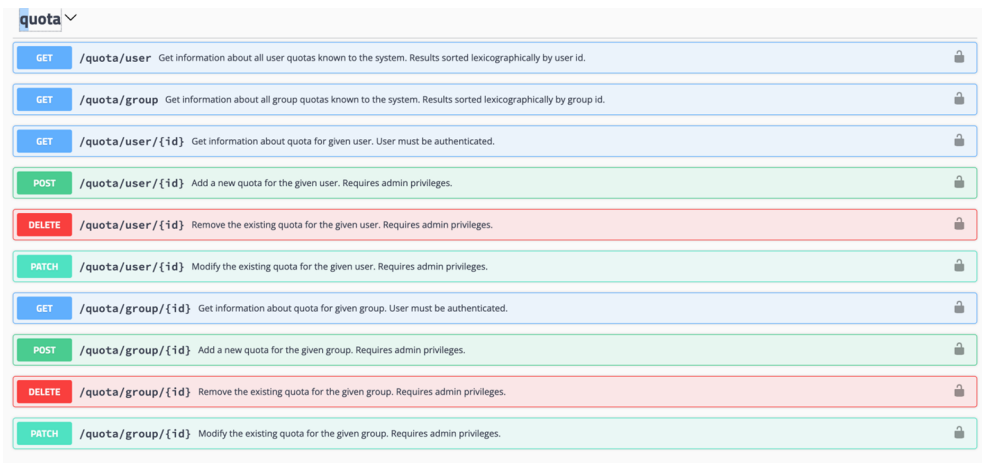
Figure 3. dCache quota REST API visualized with the help of the Swagger documentation tool.
