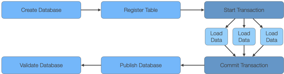
Figure 3: Schematic view of the data ingestion process into Qserv database.
