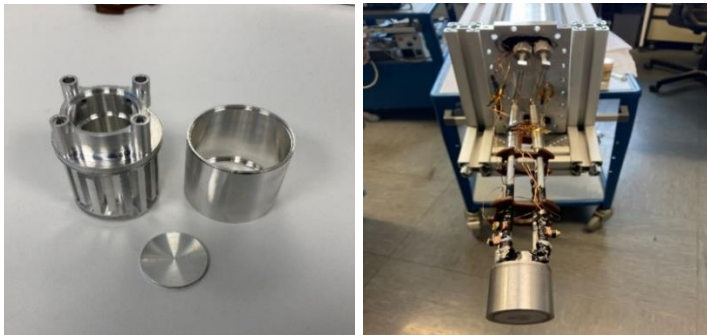
Fig. 1. Left: the moderator vessel with ethane and helium cryogenic supply lines. The helium cooling flows through the outer labyrinth. Ethane is condensed and frozen inside the inner volume. Right: a flexible mounting configuration with the moderator volume and four temperature sensors for adaptive experimental setups at the front of an extraction plug containing the neutron.
