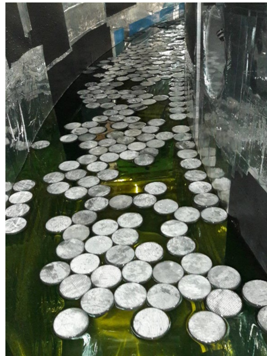
Fig. 2. View inside the flume on the water surface covered by artificial pancake ice.
