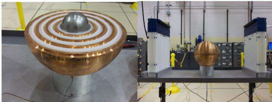
Fig. 3. Pu-Cu (also called SCRαP - Subcritical Copper-Reflected \alpha -phase Plutonium) experimental set-up. Case 7, Pu ball and 8 reflector layers: polyethylene layer followed by alternating layers of copper and polyethylene configuration (Left) and two ^3\text{He} array detectors (Right) (cf. Fig. 8 of FUND-NCERC-PU-HE3-MULT-003 in 2019 ICSBEP Handbook [3]).
