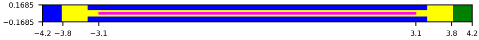
Figure 3: Top view of the system: the colors pink, yellow, blue, and green stand for enriched uranium, aluminum, water, and cadmium, respectively. The numbers are expressed in centimeters, the z-axis is limitless, and all sides have reflective boundary conditions.
