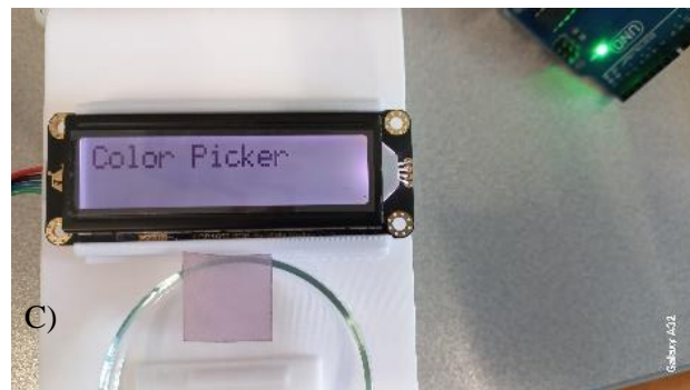
Fig. 6. Backlight of the I2C 16x2 LCD Display reproducing the color of the plasmonic paper detected by the TCS34725 color sensor.
