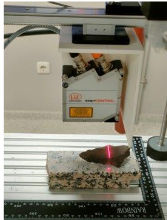
Fig. 10. Rock with engravings scanning process
