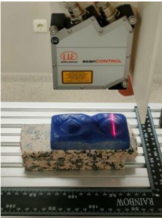
Fig. 8. Granitic stone frieze scanning process
