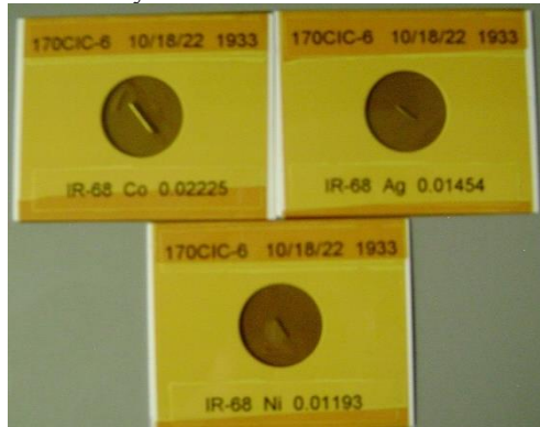
Fig. 5. Dosimeter wires were fixed within a standard geometry following irradiation.
