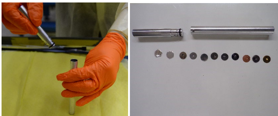
Fig. 2. (Left) An aluminum sample tube used in Godiva IV ‘glory hole’ irradiations. (Right) Foil loadout for the Godiva IV burst irradiation in this work.
