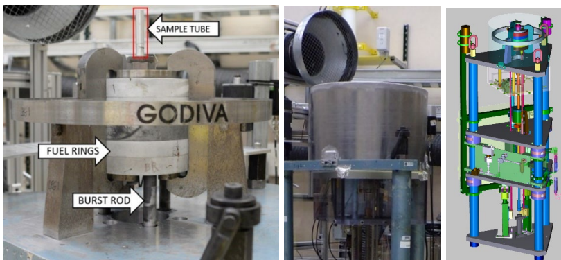
Fig. 1. (Left) Godiva IV with the ‘top hat’ removed and an aluminum sample tube inserted. (Middle) Godiva IV shown with the ‘top hat’ replaced. (Right) 3D CAD rendering of Godiva IV and associated mechanical drives and support structures.
