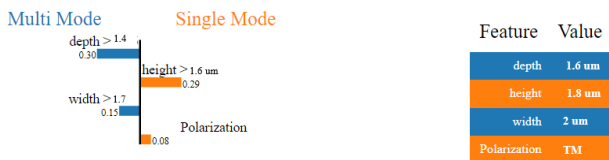
Fig. 3. Explanation of a sample prediction, with parameters and probabilities of getting SM or MM behaviour, and a sample combination of the same for a SM waveguide.
