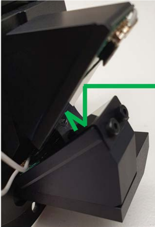
Fig. 2. Structure of a two photodiode light trapping detector.
