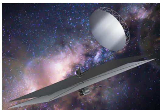
Fig. 2. 14-m diameter aperture space telescope SALTUS using inflatable off-axis primary mirror and sun shield. [2]
