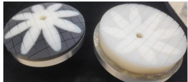
Fig. 4. 3D-printed polishing tools for a radius of 88,845 mm
