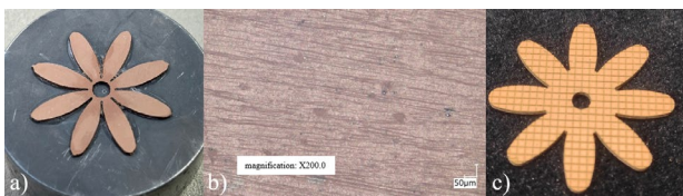
Fig. 3. Tool with cerium oxide foil, diameter of 25 mm a) pad applied to a tool body using glue b) 200x magnification of foil surface before polishing c) structured foil in a cross shaped pattern with line spacing of 1 mm and a depth of 400 \mu m
