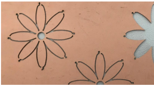
Fig. 2. Laser-cut polishing tools with a diameter of 25 mm and micro joints for better handling
