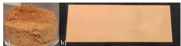
Fig. 1. a) Cerium oxide polishing powder with an average grain size of 2\mu\text{m} b) Cerium oxide foil out of polishing powder, 100mm x 40mm x 1mm
