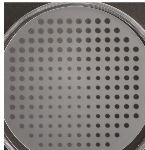
Fig. 1. Illustration of the unreproducible polishing spots on a fused silica wafer caused by the Twyman effect
