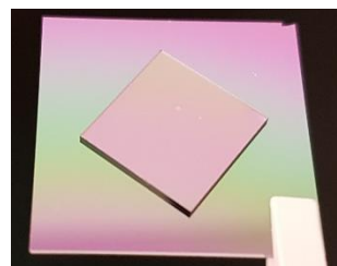
Fig. 5. Molecular wafer bonding between LN X-cut and oxidized Si samples
