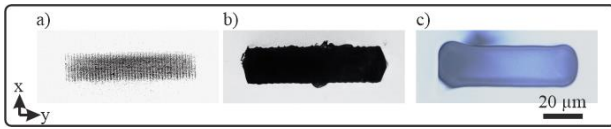
Fig. 1. Light microscope image of cross section of a) fs-laser modification, b) selectively etched channel, and c) channel after 25 h of annealing at 1060°C.
