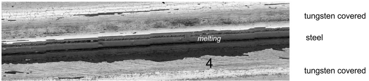
Fig. 5. Image of backscattered electrons: zoom on 4th ridge from figure 4 right, rotated by 90 deg. The steel started on the top of the ridge, where the tungsten coating is missing.
