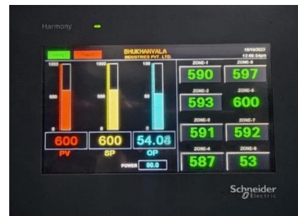
Fig. 5. Thermocouple temperature display showing maximum temperature variation of the emitter plates within 2% of the set temperature.
