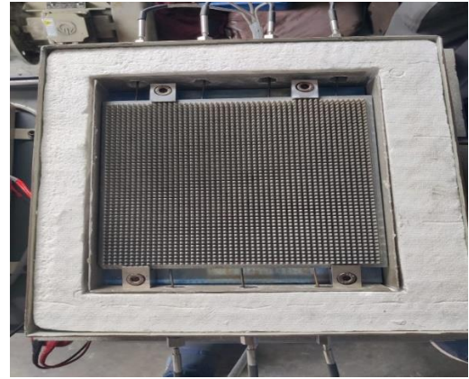
Fig. 4. Integration of heating system with emitter plate and thermocouples inside a thermally insulated box.
