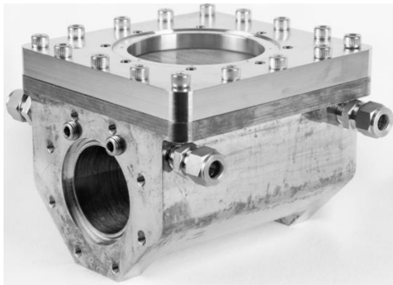
Fig. 4. Prototype vacuum pumpout with a 63.5 mm ID.
