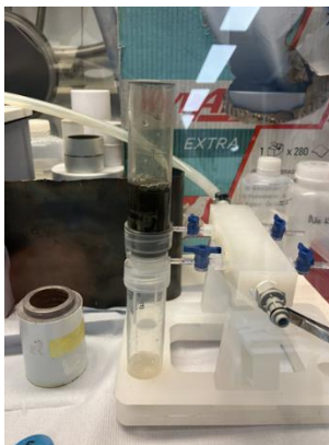
Fig. 1. A filtration setup used for the filtration of the undissolved residues
