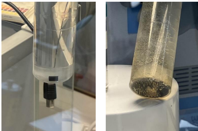
Fig. 3. Pellets dissolution in hot nitric acid, pellet before starting the experiment (left) and disintegration after 30 minutes (right)
