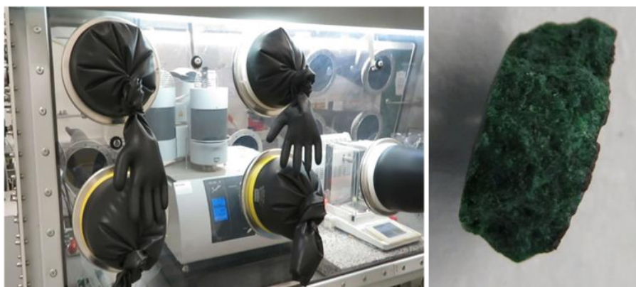
Fig. 2. Example of NNL's fuel manufacturing and characterisation capabilities – thermal analyser in argon glovebox (left) and NaF-KF-UF 4 (FUNak) fabricated at NNL (right).
