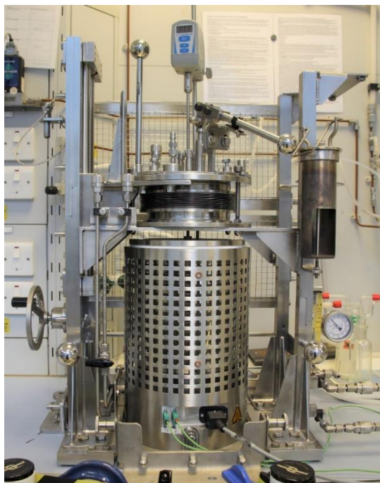
Fig. 3. The pyrochemical alpha-active processing apparatus (PAPA), has been developed to handle and investigate the electrochemical and physical properties of actinides (including Pu) in molten salt mixtures. Note that the protective heat guards have been removed in this commissioning image.
