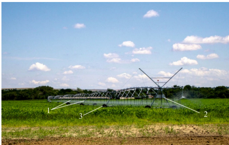
Fig. 1. General view of the irrigation machine "Kuban-LK1" 1 – support trolley; 2 – console part; 3 – pneumatic wheel.
