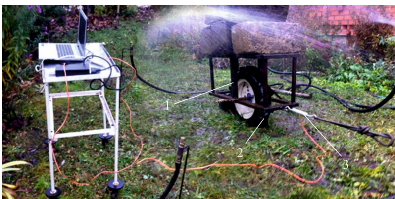
Fig. 2. General view of the experimental setup for determining the energy coupling properties of a prototype pneumatic tire of the IM: 1 - prototype sample; 2 - pneumatic wheel; 3 - strain gauge unit.
