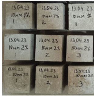
Fig. 3. Cube samples with the length of 10, 20 and 30 mm steel fibers in amount of 1.0, 2.0 and 3.0 %.
