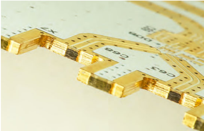
Fig. 4. An example of metallization of the end of a hybrid printed circuit board.
