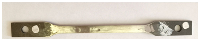
Fig. 1. Example of a flat sample for low cycle fatigue tests.
