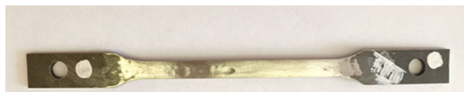
Fig. 2. Corrosion rate measurement points.
