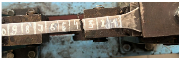
Fig. 9. Destroyed sample and destruction zone.
