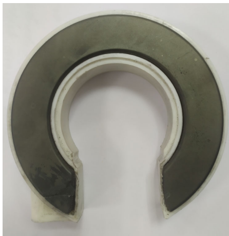
Fig. 4. The magnetic part of the sensor element.
