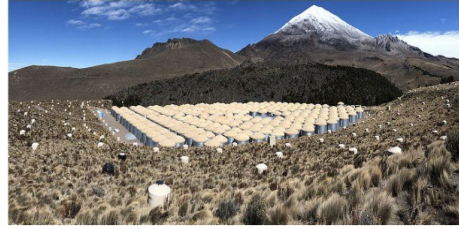
Fig.1. Photograph of the HAWC observatory taken from the base of Sierra Negra with Pico de Orizaba in the background. The 300 large main array WCD tanks are in the center. The smaller tanks seen in the photo are those of the outrigger array.
