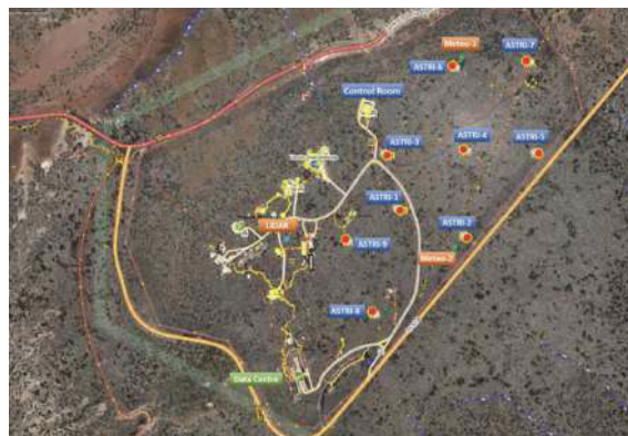
Figure 1. Positions of the 9 telescopes of the ASTRI Mini-Array. The picture shows the positions of the 2 meteorological towers, LIDAR, transformer station, local control room, and data center. (from [9]).
