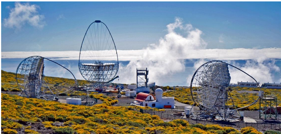
Figure 1. The IACT telescopes at the Roque de los Muchachos Observatory, left to right: MAGIC-2, LST1 and MAGIC-1. One can see that the telescopes are above the cloud cover over the Atlantic ocean. In the middle of the picture one can see the experimental building, where the dome above the roof houses the micro-LIDAR instrument. The latter regularly measures the transparency of the atmosphere.
