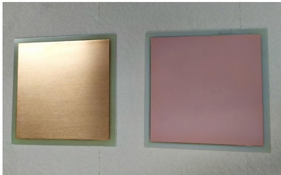
Figure 4. Pictures of the anode plate before (left) and after (right) \text{TiO}_2 coating.
