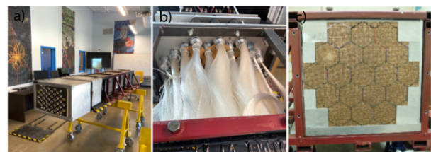
Figure 1. The original DREAM calorimeter before reconfiguration: (a) with the PMT readout box, (b) large scintillating and clear fiber bundles behind the absorber, and (c) the transverse segmentation with 19 hexagonal towers. The tower size is r \approx 3.71 \text{ cm} .
