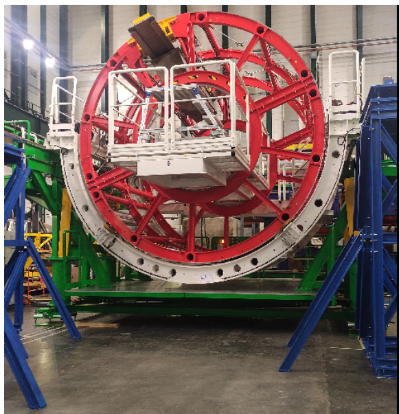
Figure 5. ECAL new supermodules extraction and insertion tool Enfourneur E2.
