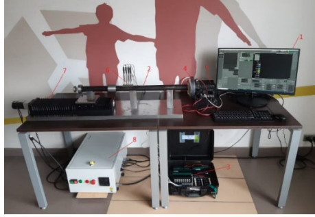
Fig. 3. General view of MAI interferometer installation (impedance tube) with normal incidence of sound waves for studying the acoustic characteristics of sound-absorbing materials and structures: 1 – personal computer, 2 – impedance tube of 30 mm in diameter inside which the test sample is located, 3– recorder type Ecophysics-500, 4 – loudspeaker with frequency range 0.5 – 20 kHz, 5 - power amplifier with built-in generator, allowing you to set sound pressure levels up to 160 dB, 6 - four ¼ inch pressure microphones with preamplifier (frequency range 1.6–20000 Hz, sensitivity 50 mV/Pa), 7 – linear actuator, 8 – control unit.
