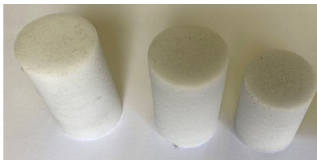
Fig. 9. Samples of "EKOHOR" sound-absorbing material of various heights of 50, 80 and 100 mm with a diameter of 30 mm for research at the MAI “interferometer” installation.
