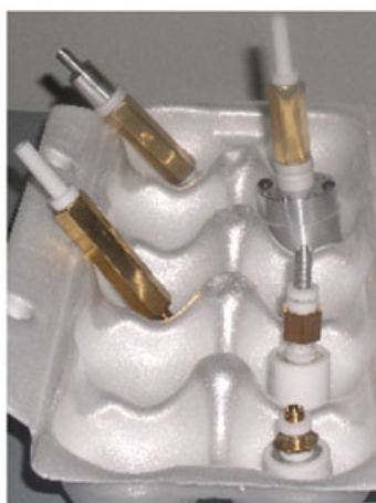
Fig. 2. Various designs of resonator cells with test samples.
