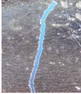
Fig. 5. Image of a film defect obtained using an optical microscope.
