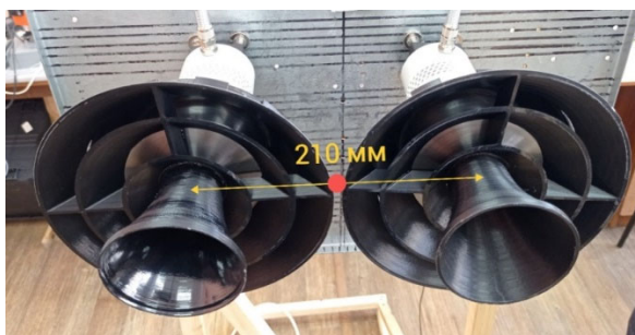
Fig. 11. Two directional ultrasonic emitters with reflectors and horns.
