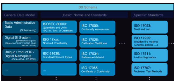
Fig. 5 : Structural view of norms and standards underlying the DX-schema, advanced version of [2], Fig. 7 ©Creative Commons Attribution 4.0 license
