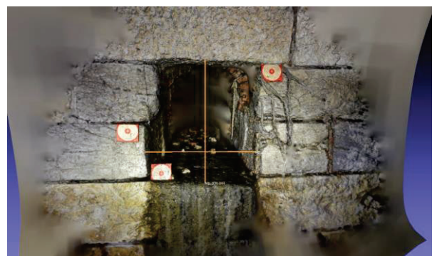
Fig. 4. Sewer's digital model, showing the measurement of its cross-section dimensions.
