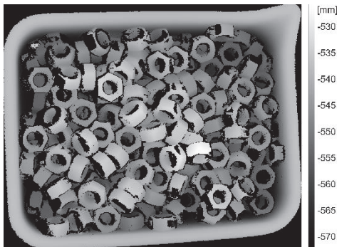
Fig. 1. Example of a depth image acquired with the SUT.
