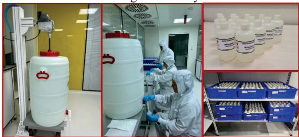
Figure 5: Homogenisation and bottling in ISO Class 6 Clean Chemistry Laboratory at TÜBİTAK ÜME
