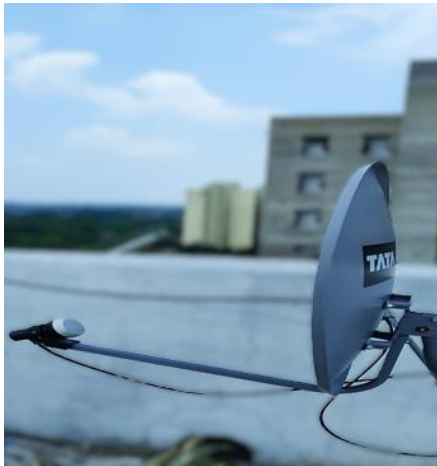
Fig. 3a. Radio telescope at angle of inclination 20°
