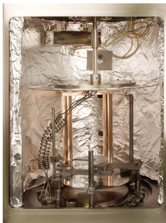
Fig. 4. View of the applied thermal deposition setup, Edwards AUTO 306®. The quartz lamp is situated above the evaporation wheel, the tantalum crucible is clamped between the massive copper electrodes below the evaporation wheel.
