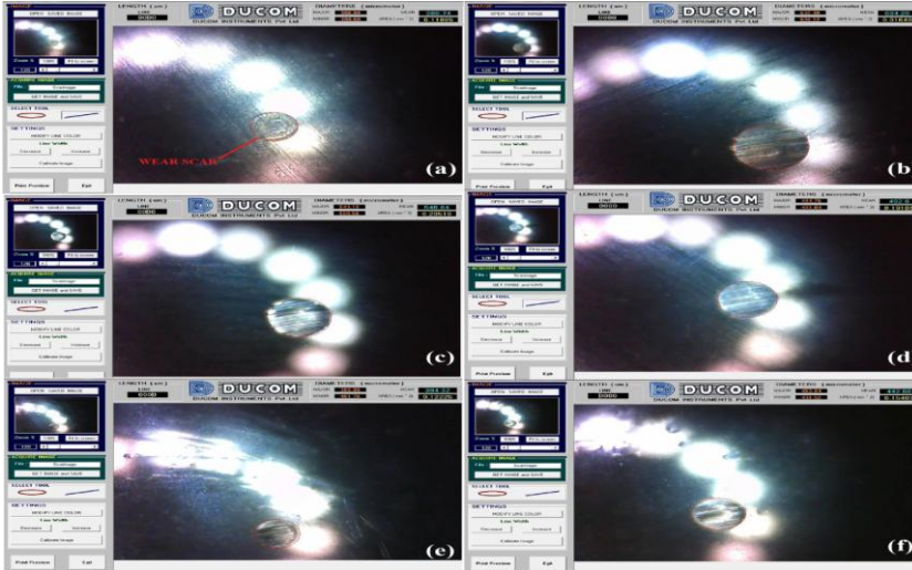
Fig. 2. Wear scar diameter of (a) Without Field CNSO + 2.5wt% TL (b) CNSO + 1wt% TL (c) CNSO + 1.5wt% TL (d) CNSO + 2wt% TL (e) CNSO + 2.5wt% TL (f) CNSO + 3wt% TL
