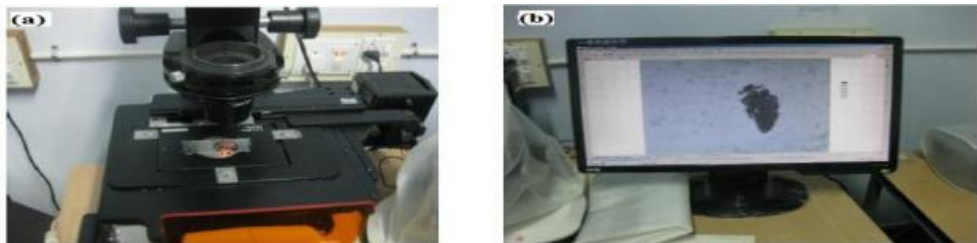
Fig .2 a) Microscope analyser (b) Microscope image of cross-sectional area of VGF
