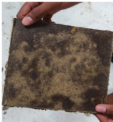
Figure 5. Fabricated Eco-Friendly Hybrid Composite Panel Using RiceHusk, RiceHusk, Groundnut Santa Maria Feverfew
